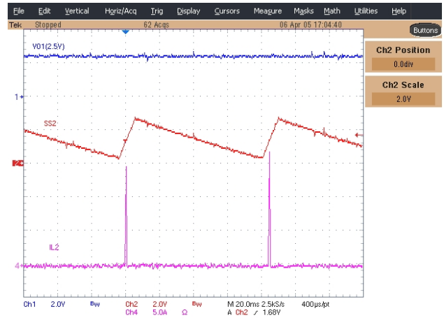
Figure 14 - 1.8V output shorted Ch1: Vo1, Ch2: SS2, Ch3: Inductor Current
