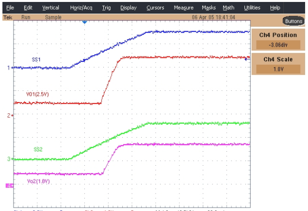
Figure 16 - Prebias Start up Ch1: SS1, Ch2: Vo1, Ch3: SS2, Ch4: Vo2
